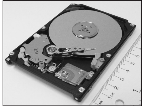
Inside of a typical hard disk drive used in a laptop computer. | Photo by S. Kasap.
