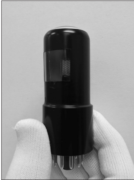
A photomultiplier tube (Hamamatsu R5108) that is used in near infrared spectrophotometers and luminescence measurement applications. The light entry window is on the left and the tube is painted black to eliminate light reflections in the spectrophotometer. The photocathode is Ag-O-Cs with a useful spectral response range over 400 – 1200 nm. The tube has 9 dynodes to generate a multiplication gain up to 10^6 .
