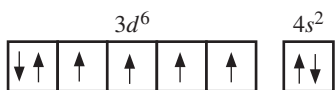
Figure 8.18 The isolated Fe atom has four unpaired spins and a spin magnetic moment of 4\beta .
