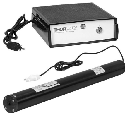
A modern He–Ne laser with its power supply. This unit provides a linearly polarized TE 00 output at 633 nm (red) at a power of 10 mW. The beam diameter is 0.68 mm and the divergence is 1.2 mrd. | Courtesy of Thorlabs.
