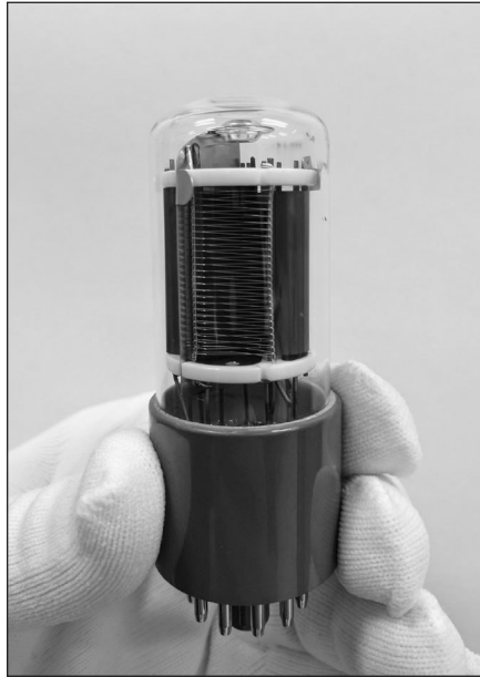
A photomultiplier tube (Hamamatsu 1P21) for the detection of low-level light in the visible range. The photocathode is Sb-Cs with a useful spectral response over 300 – 650 nm. The tube has 9 dynodes and a typical multiplication gain of 6 \times 10^6 . This particular model has the advantage that its dark current is small, which increases the signal-to-noise ratio capability of this photomultiplier tube.
