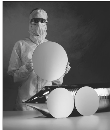
Above: 200 mm and 300 mm Si wafers Left: Silicon crystal ingots grown by the Czochralski crystal drawers in the background. | Courtesy of SunEdison Semiconductor.
