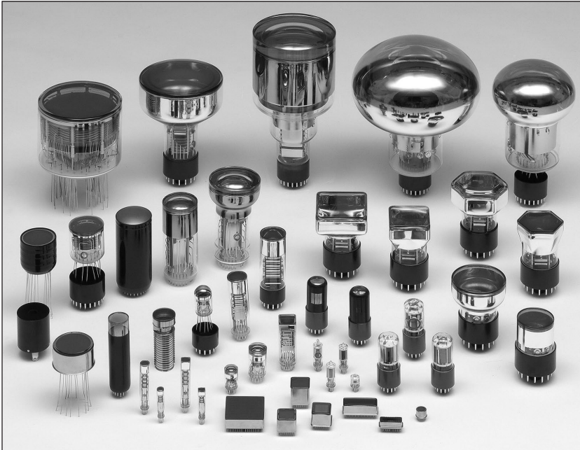
Photomultiplier tubes rely on the photoelectric effect and secondary emission. | Courtesy of Hamamatsu.
